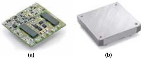
Figure 1. Pictures of an open-frame module (a), and a potted module (b).
