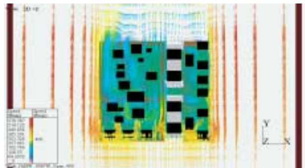
Figure 4. Air velocity vector map for an open module at 2 m/s (400 ft/min)
